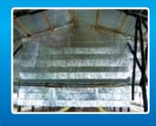
Lateral curtains are placed inside the shed in the chicken reception area. Their main goal is to maintain the inside temperature controlled during the first 12 breeding days, when gas is used to keep a temperature of 90° f.
