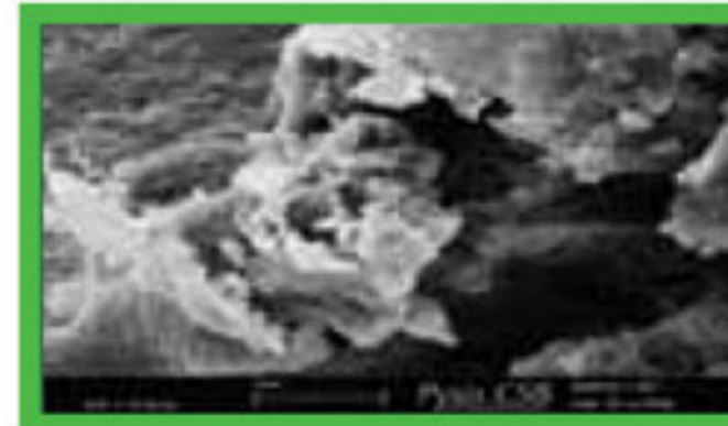
Biomass-consuming colonies of bacteria and fungi grow in polymer cracking areas
